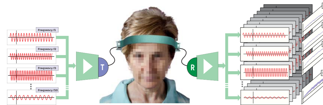
Fig. 1 An outline of the process of forming multidimensional phase bundle: The compound multi-spectral signal is being emitted at one side of a patient's head and after transverse skull bones and the brain tissue it is being received on the other side
